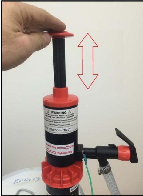
Note: You do not need to greatly pressurize the pump / drum to dispense. The number of 'pump cycles' required will depend on the volume of liquid in the drum.
