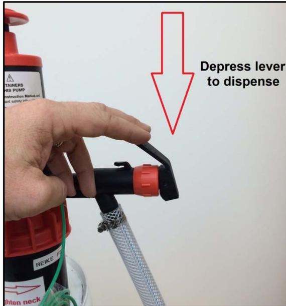
Note: If the pressure is insufficient to dispense, if liquid does not flow, 'pump' the piston handle a few more times. Do not overpressurize.
